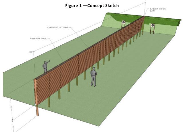
The Contractor shall supply the labor, equipment, and material to construct this partition.
